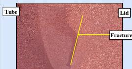
Macrograph of the transverse section of the FSW weld. Fracture occurred at the line of entrapped oxide particles (marked by a yellow line).
