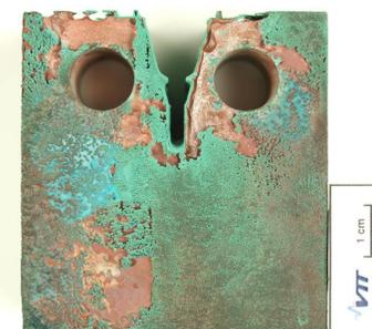
Fig. 4. Extensive general corrosion in the CT specimen after 4400 h (90°C) in aerated simulated Olkiluoto groundwater
