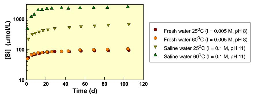
The dissolution of montmorillonite was modelled with TOUGHREACT, so that the salinity of waters was taken into account. Modelling results were compared with the experimental result. The comparison of pH results (see below) reveals the need for development of the models.
