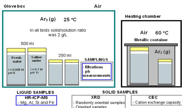
The elemental concentrations of ultra filtrated solution samples were analysed with high resolution inter coupled plasma mass spectrometer (HR-ICP-MS). The purified montmorillonite and the solid material gained from experiments were analysed with XRD (X-ray diffraction) at ERM (Etudes Recherches Matériaux) in Poitiers, France.
