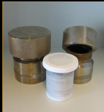
Teflon reactors used for kaolinite synthesis
