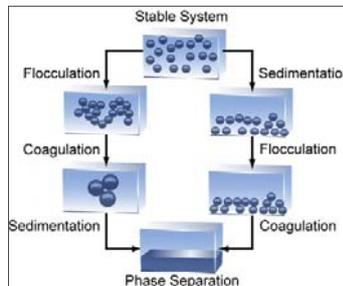
Fig. 2. Processes that deal with the stability of colloidal systems by DLVO theory (Derjaguin, Landau, Verwey and Overbeek)
