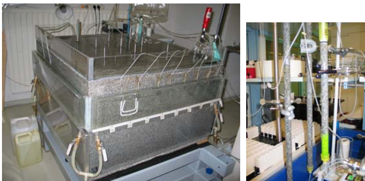
Fig. 1. Set-ups for radionuclide migration experiments; Kuru grey granite block (left) and core columns (right).
